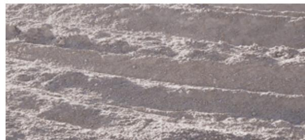
As a result of the extrusion process, pieces have a natural, laminated and homogeneous, structure providing higher resistance and durability than in dry pressed products. This structure is defined by the relationship between the extrusion process and the mixing of different raw materials and their granulometry.
